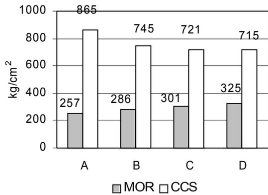
**Fig. 2 CCS and MOR data of sintered samples.**
