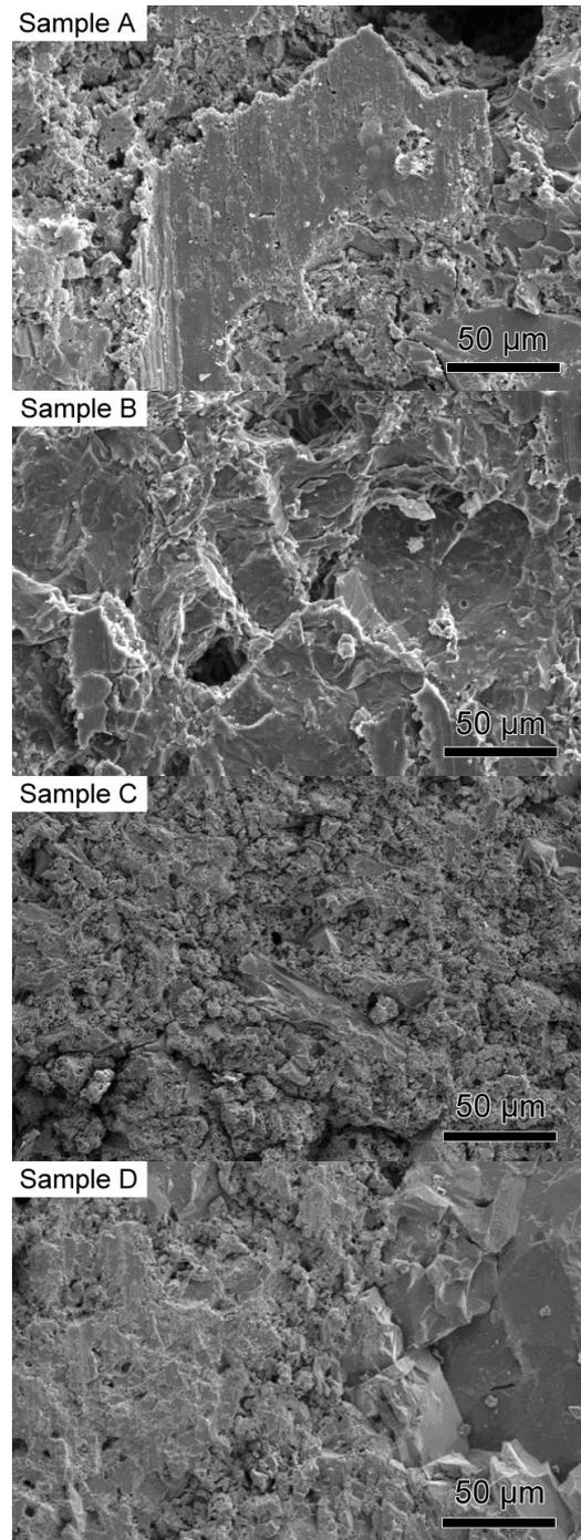
**Fig. 5 SEM micrographs of 1450°C sintered bodies.**
