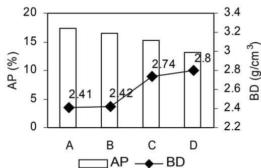
Fig. 1 Bulk density and apparent porosity of sintered samples.
