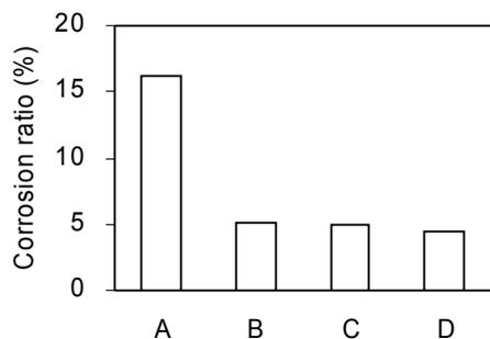
**Fig. 4 The corrosion ratio evaluated by static slag crucible method (1450°C).**
