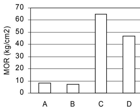
**Fig. 8 MOR data after thermal shock testing (1000°C, water quenched, 6 cycles).**
