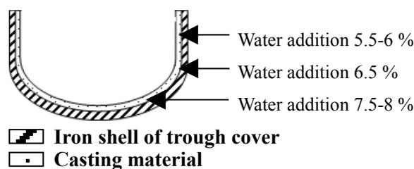
**Fig. 9 Working condition of castables on trough cover.**
